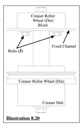
4. Hold the assembly in position and tighten the bolts, (**J**) to hold the block in place. Turn the hub and make sure the hub surface aligns with the centerline completely. Also make sure that the wheel is directly behind the blade assembly. A line from the blade shaft to the die shaft must be perpendicular to the channel front face.
