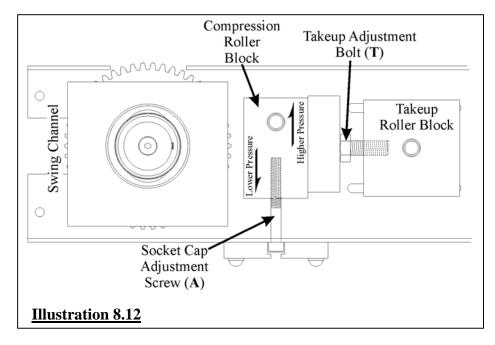
9. You may wish to test a few bags with the heaters "OFF". Then test the compression roller settings with the heater "ON". Be sure to allow the manifold to heat up completely before testing begins. Follow the guidelines mentioned in the Quality Control section of this manual to determine a good seal.
