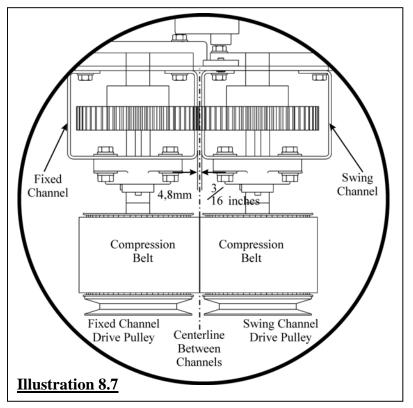
allow the roller to move. Loosening the screw too much will allow the screw (shaft) to skew too much to accurately align the compression belt.
