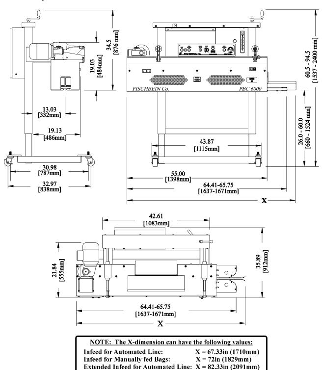
Air Consumption Minimum Requirement: 420 SCFH (11,9 SCMH) Air Pressure Requirement: 90 PSI (6,2 bar) (with ½ inch air line)
