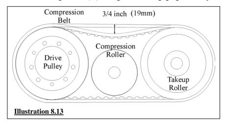
11. To adjust the compression rollers refer to "ADJUSTING THE PRESSURE BETWEEN THE COMPRESSION BELTS" page 32.
