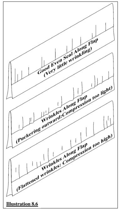
two types of wrinkles that can appear to suggest an adjustment is needed. Wrinkles that are present, but NOT pressed flat, indicate that the pressure between the belts is too small and needs to be increased by bring the rollers closer together. The second type of wrinkle is large and pressed flat into the flap. This flat wrinkle indicates that the pressure is too large and needs to be reduced.
