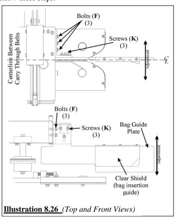
Make further adjustments to the guide as needed when the electrical system is "OFF". Refer to the Quality Control section of this manual to determine proper bag closures.
