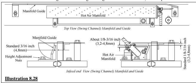
contact with the manifold and the glue will begin clogging the holes in the manifold top. Obstructed holes prevent the hot air from exiting the manifold and will not allow the glue strip to completely heat.
