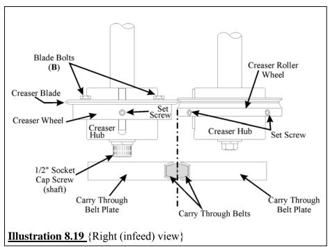
The creaser assembly must create the crease at the correct height in relation to the folder and glue line. There is a specific sequence for adjusting the setting for the creaser.
