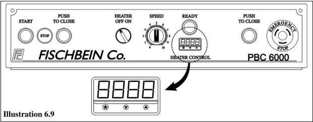
Since the bag and glue take time to heat up, the faster the system is required to seal bags, the higher the temperature setting must be. Keep in mind that every time the conveyor and machine speed is changed the temperature should be changed. Leaving the temperature set higher than needed for a new setting, my cause the bag or glue to char. THIS IS A FIRE HAZARD AND MUST ALWAYS BE AVOIDED!
