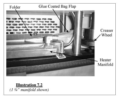
After the manifold, the folder continues bending the heated flap another 90° to complete the fold. The adhesive begins to make contact with the outer bag surface as the fold is completed and the bag enters the compression area ofthe wide machine. The compression belts guide the bag top between the compression belts. The belts press the flap firmly against the bag, to force the adhesive to penetrate the bag fibers. The completed fold and compression yield a sharp, clean fold with a strong bond.
